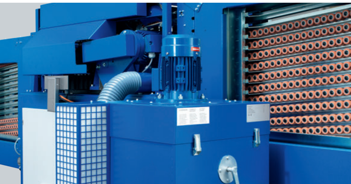
supergrinder view from the back with supplied suction device and large universal loading magazine
